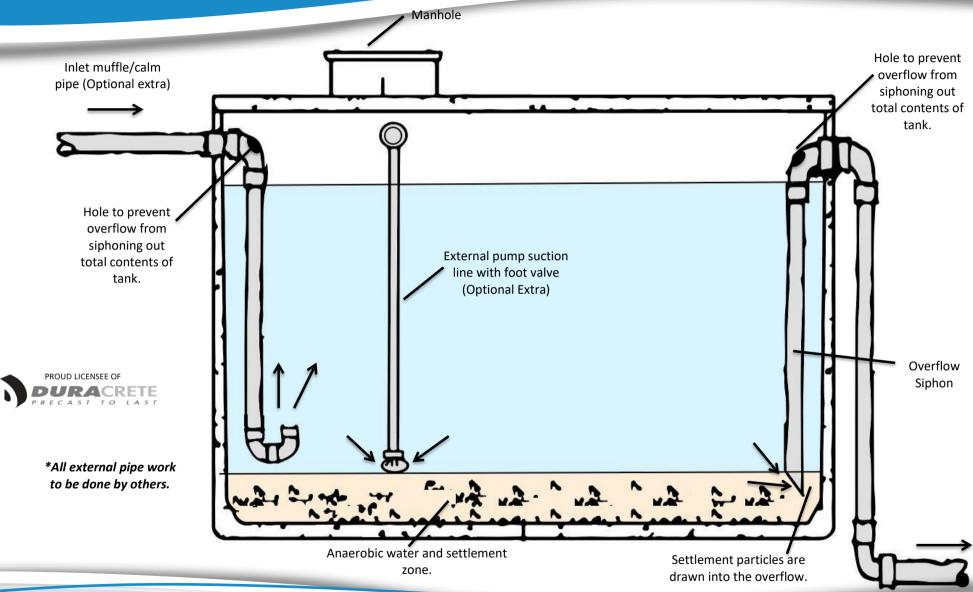
PLEASE NOTE: THE ABOVE DIAGRAM HAS BEEN DESIGNED AS A REFERENCE ONLY. ITEMS SUCH AS THE INLET MUFFLE PIPE, FLOATING OUTAKE AND THE ADAPTER PIPE DO NOT COME STANDARD WITH THE TANK; THEY ARE ADDITIONAL EXTRAS. THIS REFERENCE WAS DESIGNED TO PORTRAY THE RECOMMENDATIONS SET OUT BY BRANZ. THIS ILLUSTRATION IS NOT ACTUAL SIZE OR DIMENSIONS.
