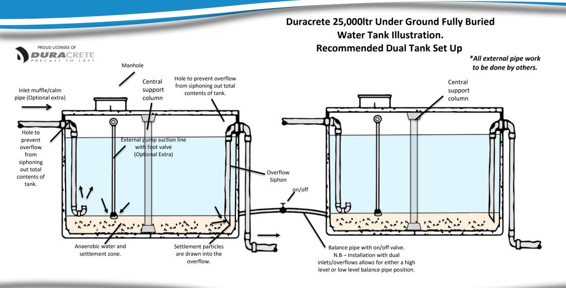
PLEASE NOTE: THE ABOVE DIAGRAM HAS BEEN DESIGNED AS A REFERENCE ONLY. ITEMS SUCH AS THE INLET MUFFLE PIPE, FLOATING OUTAKE AND THE ADAPTER PIPE DO NOT COME STANDARD WITH THE TANK; THEY ARE ADDITIONAL EXTRAS. THIS REFERENCE WAS DESIGNED TO PORTRAY THE RECOMMENDATIONS SET OUT BY BRANZ. THIS ILLUSTRATION IS NOT ACTUAL SIZE OR DIMENSIONS.
